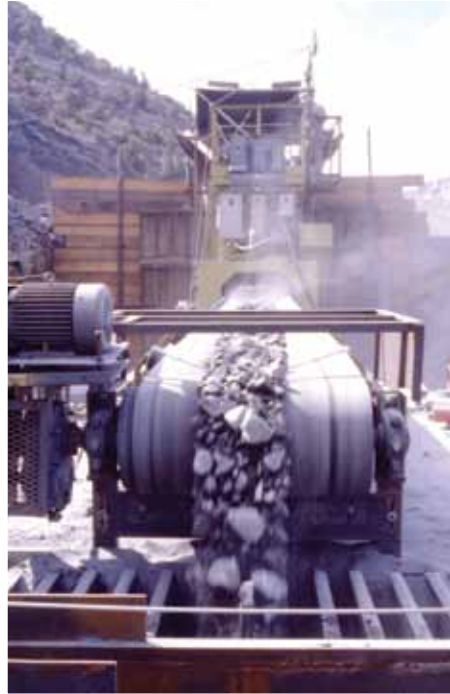
This rock crusher at the mouth of Kingston gold mine breaks rocks to a size that will pass through the grizzly or grate. They fall down a bore hole to a conveyor which carries the ore to the truck loading area.
